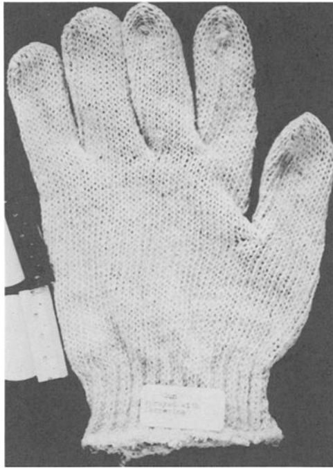
FIG. 3—Iron stains left on a glove by a revolver as revealed by spraying with 0.1% w/v ferrozine solution.
