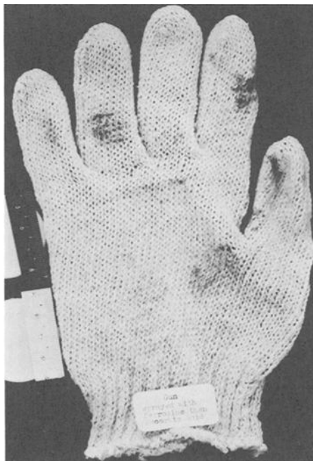
FIG. 4—Same as Fig. 3, but the stains were revealed by spraying with 0.1% w/v ferrozine solution and then 3% w/v ascorbic acid solution.
